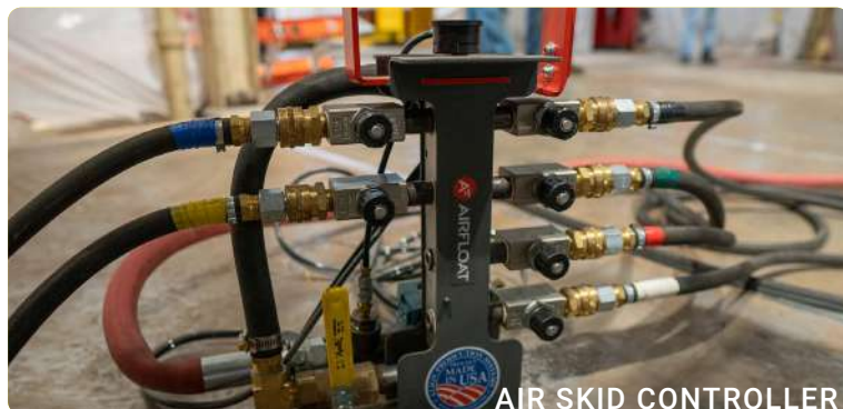
AIR SKID CONTROLLER
