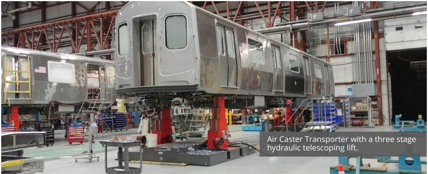
Air Caster Transporter with a three stage hydraulic telescoping lift.
