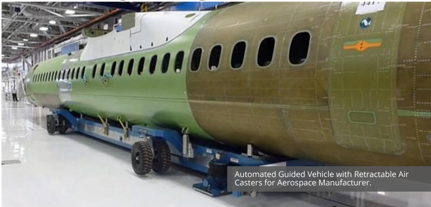
Automated Guided Vehicle with Retractable Air Casters for Aerospace Manufacturer.
