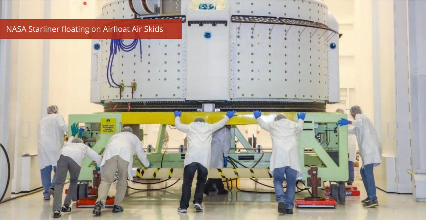
NASA Starliner floating on Airfloat Air Skids
