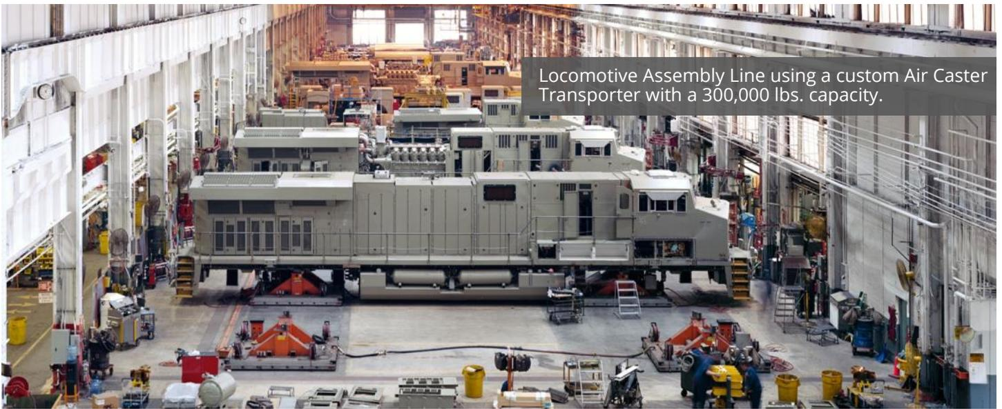
Locomotive Assembly Line using a custom Air Caster Transporter with a 300,000 lbs. capacity.
