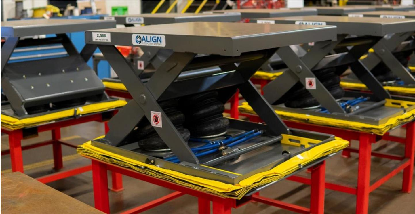
Pneumatic Lift tables are built to withstand the demands of manufacturing. All of our tables feature solid steel cross arms, and are engineered for optimum performance, strength, and durability unsurpassed in the industry. All scissor lifts meet the ANSI MH29.1-2012 design standards. In addition to standalone operation, our lift tables can be integrated into a solution with other equipment.
