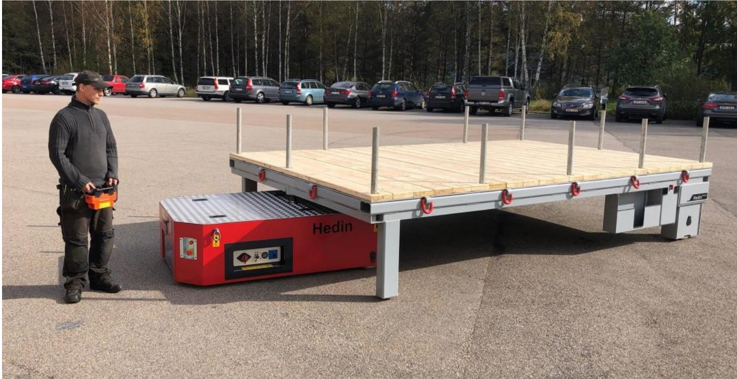
GT Tuggers give operators the ability to move materials around a plant via Remote Control, allowing for maximum control over the load. GT Tuggers can also be equipped with AGV guidance systems, enabling them to operate without the need for an operator to input movement. Our tuggers are built to lift up the front end of wheeled carts and trailers, distributing the heavy load evenly - making it effortless to move up to 220,000 lbs.
